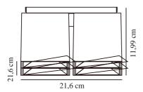
Voltage (V): 230 Volt IP degree: IP20 Maximum bulb wattage (W): 4x50W
