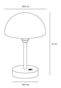
Voltage (V): 3,7 Volt IP degree: IP44
