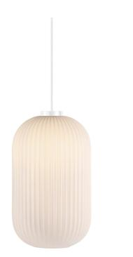
Voltage (V): 230 Volt IP degree: IP20 Maximum bulb wattage (W): 40W Class (Class 1, Class 2, Class 3): Class 2 (Double isolated) Socket type: E27 Dimmerable: Yes with compatible bulb
